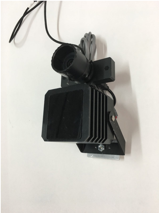
IR light is held onto the metal plate by a single screw.
