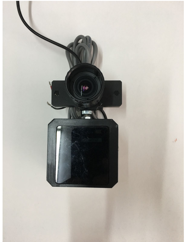
The camera's set screw has two nuts to prevent rotation.
