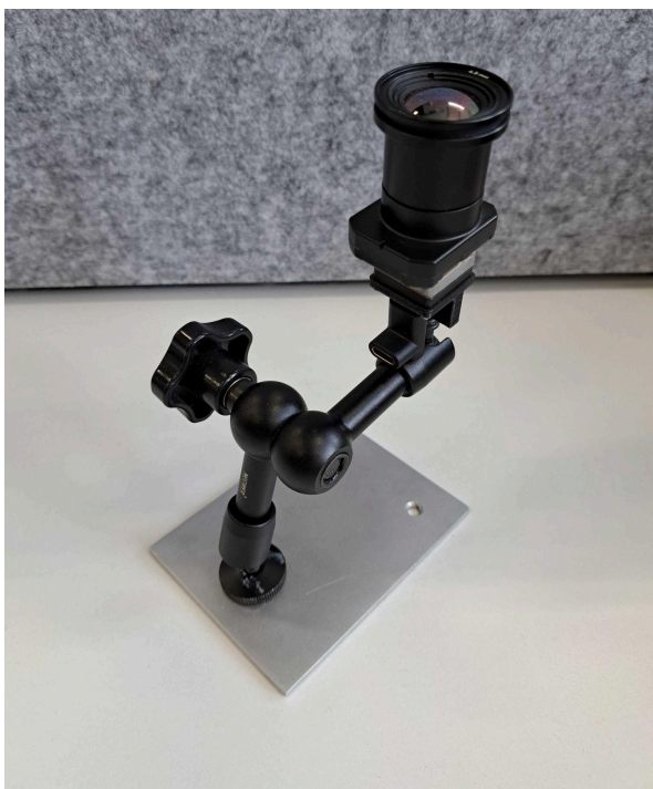
Fully assembled bracket, arm and camera
