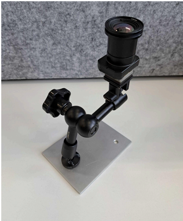
Fully assembled bracket, arm and camera
