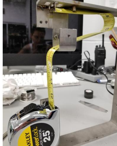
9. Finally, unscrew the tape from the metal frame by unscrewing the 2 screws holding it in place as shown here.
