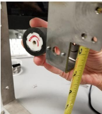
8. To change the tape, you need to bend it around in the structure in order to be able to take it out. See pictures below to help you out. Be careful not to bend the tape more than needed as it may snap and rip.
