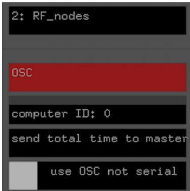
*computer ID* : the master computer will be set to 0 and the subsequent (slave) computers should be ID'ed 1, 2, etc.
