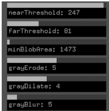
*minBlobArea* : This is the minimum size blob the Kinect will consider to be a valid target for triggering tapes. By adjusting this setting we make sure small objects such as things on the floor, light fixtures etc. will not trigger the piece.
