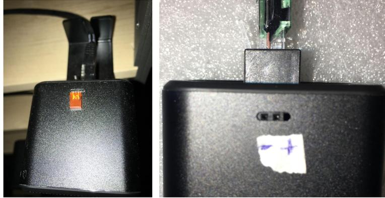
When looking at it from the front, the negative entry (-) is on the left and the positive (+) entry (+) is on the right.
