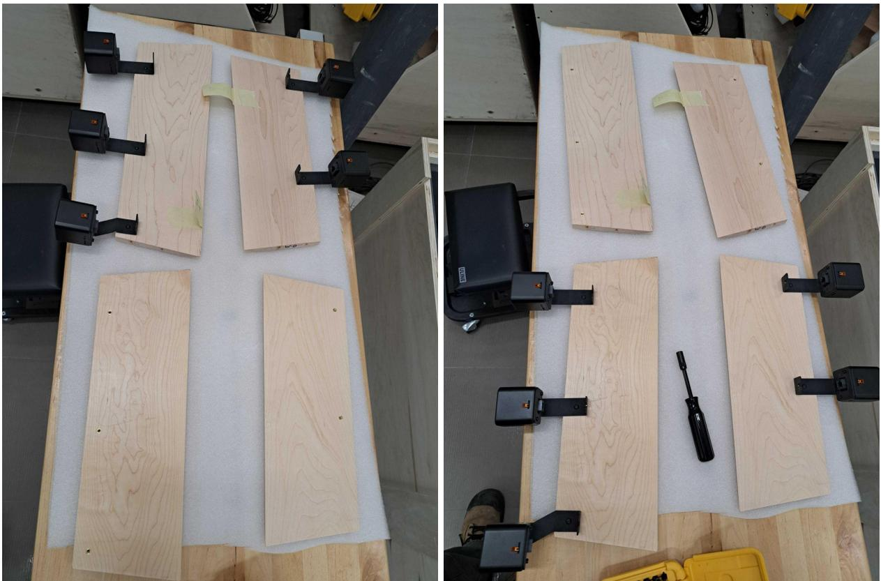
Mount the new wooden slat back onto the metal slice in the sphere, following the same process as when it was initially removed. Take care not to overtighten the wood screws, as excessive force damages the slat.
