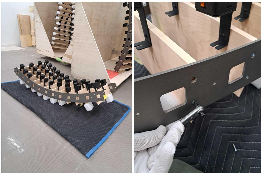
Each row of the sphere contains a different model of slat and each individual slats has unique speaker anchoring hole positions. Consequently, the provided spare slats do not have their brass inserts or holes premade.
