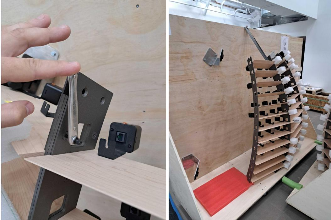
Next, gently place the slice on its back, ensuring it rests on the provided foam cubes. It is crucial to avoid applying additional weight to the part to prevent damage to other wooden slats.
