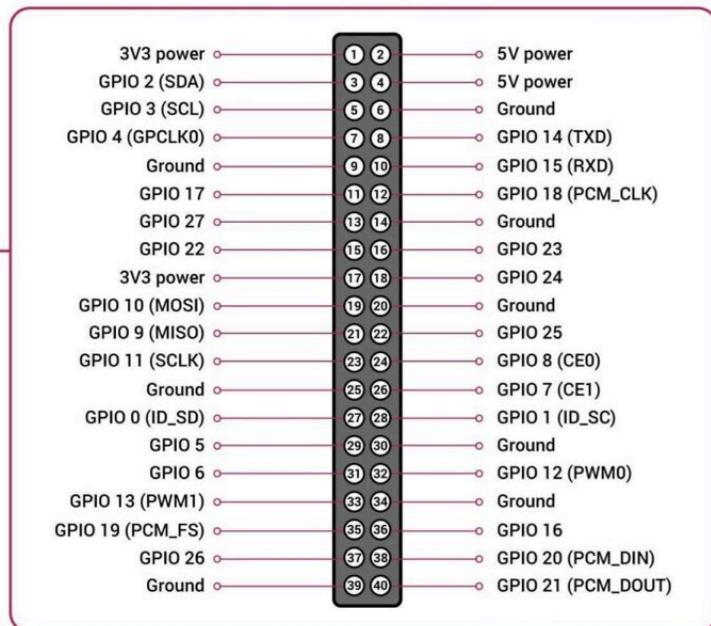
**40 GPIO Pins Description of Raspberry Pi 5**
