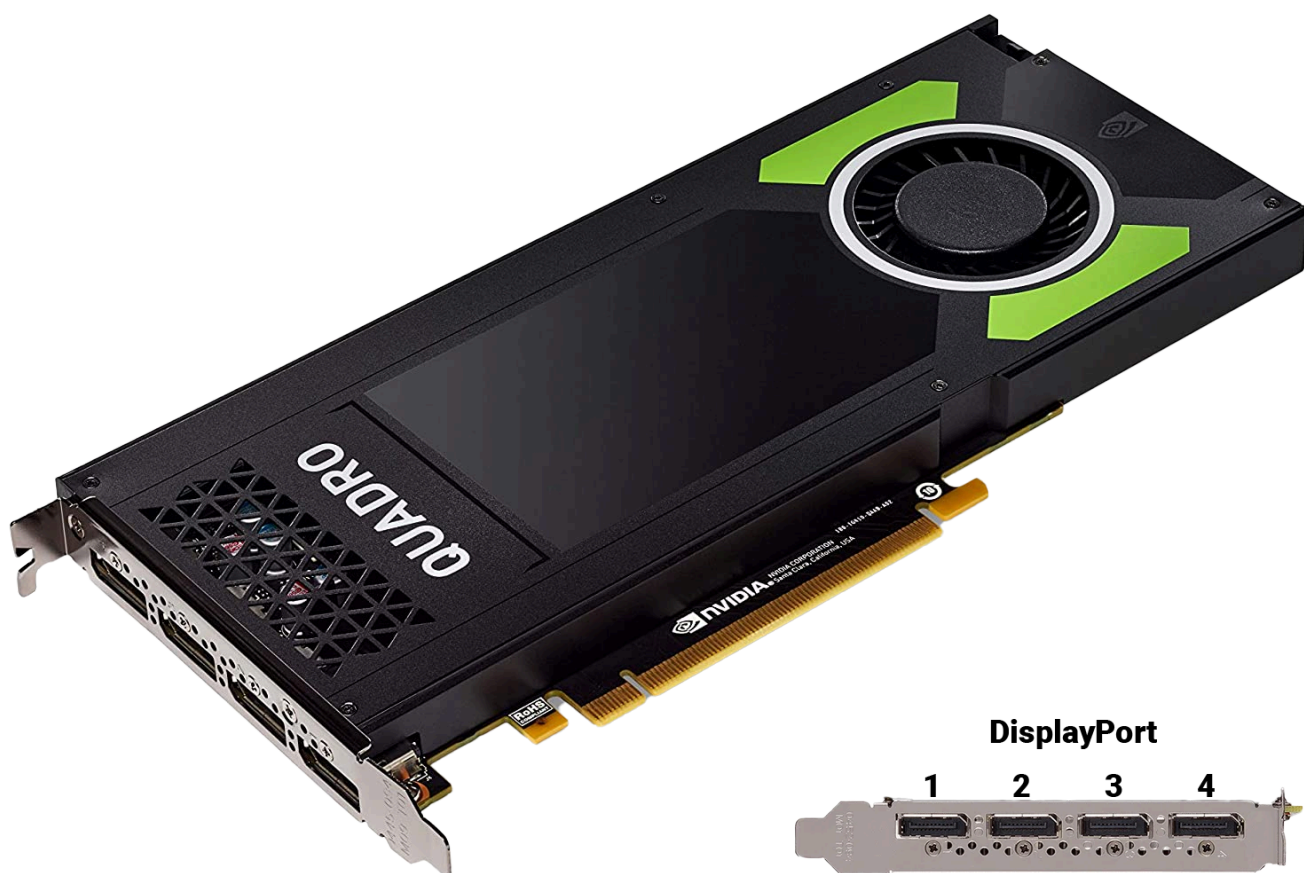
nVidia Quadro P4000 w/ DisplayPort layout
