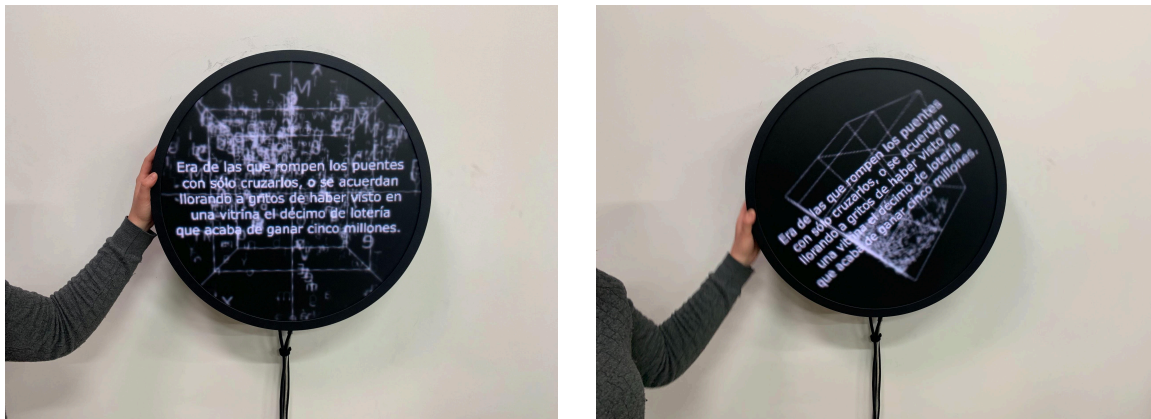
Left: Text properly centred; Right: Text askew, calibration needed.
