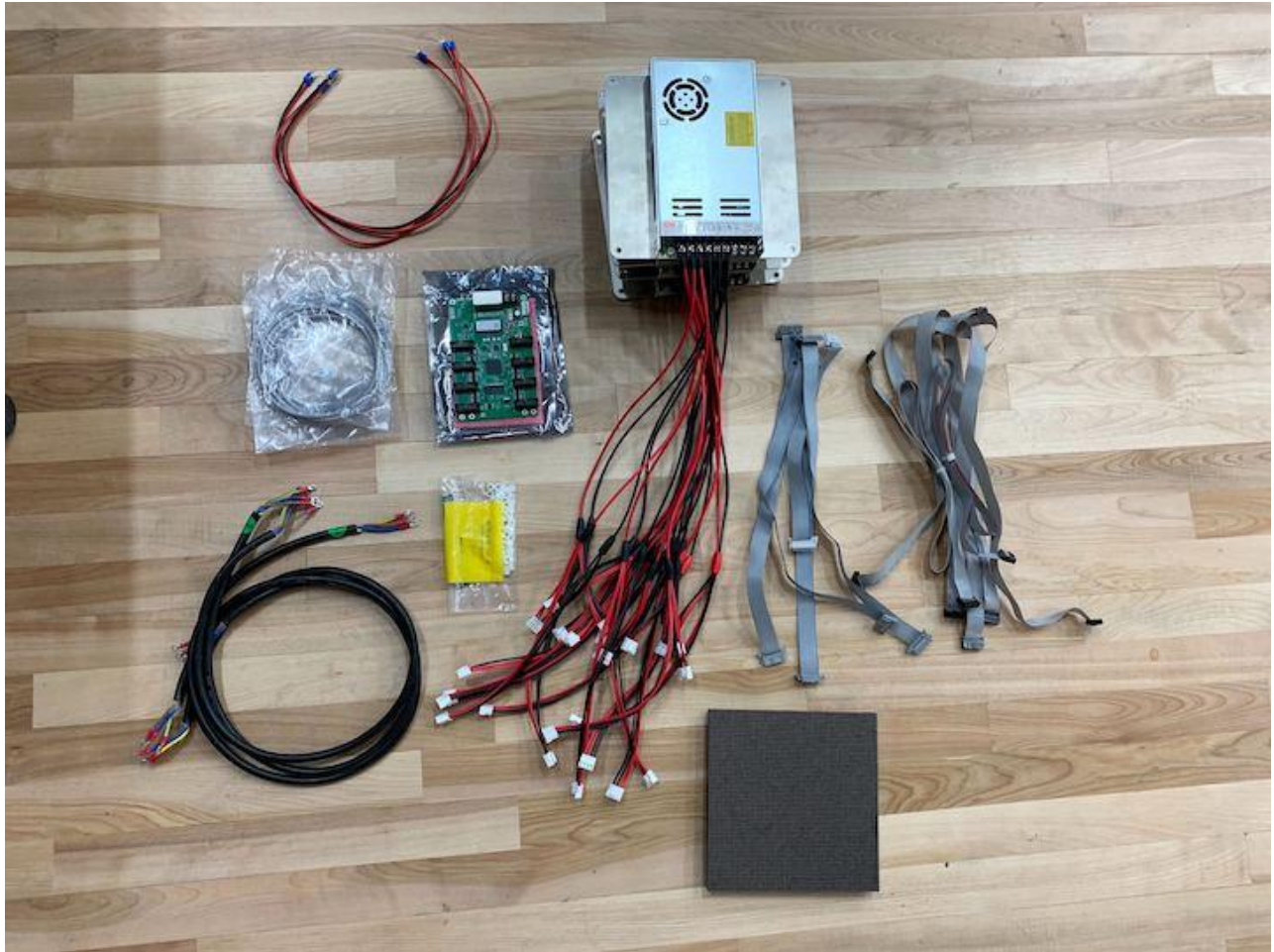
For consultation: Power Supplies, Custom PCB Boards, Custom LED Panel, and respective cabling.
