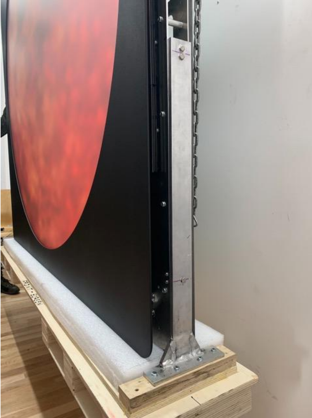
Bracket attached to the base of the crate, which keeps the display stabilized and upright.
