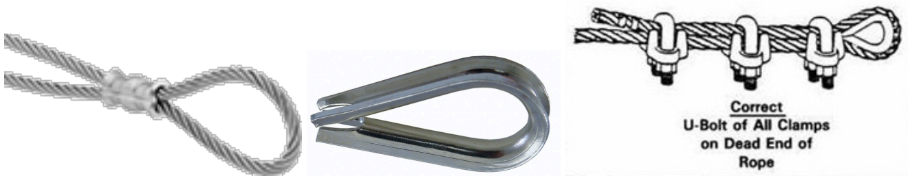
Accepted rigging (NOTE: Always use thimbles to avoid damage)
