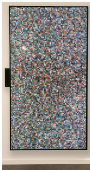
Portrait mode, with depth sensor on the left side with display smaller than 75"
