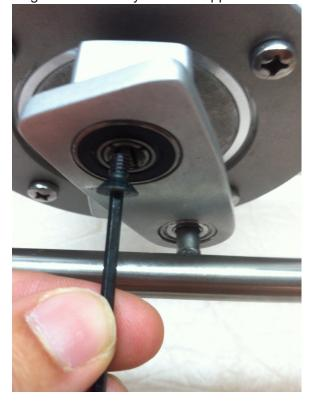
Be careful not to put thread locking liquid on the bearings.
