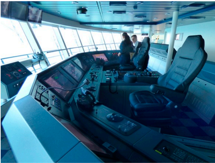
The horseshoe-shaped main bridge console.
